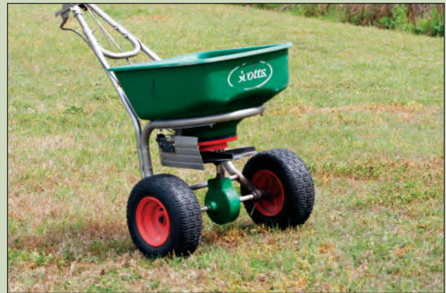
A deflector shield directs fertilizer away from your maintenance-free zone.
