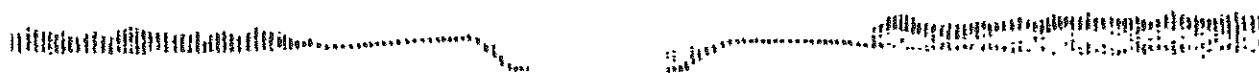
Figure 7. This is the vertical profile of a transect from harvested canopy to crop cover (illustration above from the left going to right). There are less second returns (red) than the 2017 LiDAR. This indicates that the platform and/or sensor used for 2023 Pilot Project is not desirable. In the middle is the ditch (water filled) and on either side the dykes. Note - that there are practically no second returns from the bare soil, only first returns.
